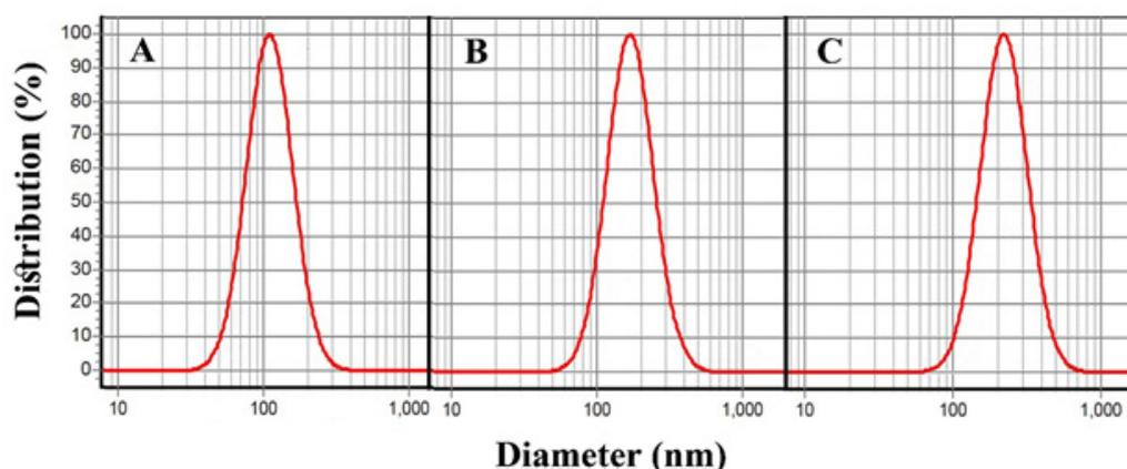
**Figure 1.** The hydrodynamic diameter of A) chitosan nanoparticles  $111 \pm 7$  nm, B) chitosan nanoparticles containing *C. verum* EO  $161 \pm 6$ , and C) chitosan nanoparticles containing cinnamaldehyde  $218 \pm 11$  nm
