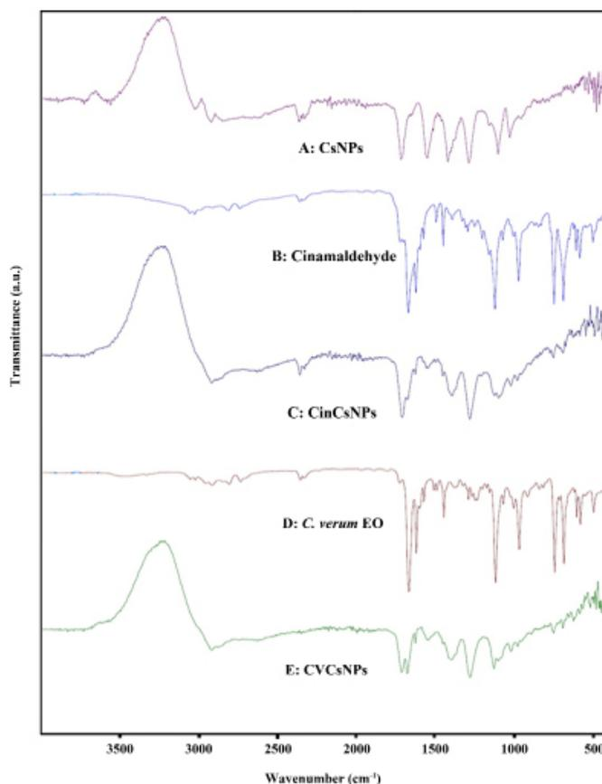
**Figure 3.** Confirmation successful loading of *C. verum* EO and cinnamaldehyde in chitosan nanoparticles; A) chitosan nanoparticles, B) cinnamaldehyde, C) chitosan nanoparticles containing cinnamaldehyde, D) *C. verum* EO, and E) chitosan nanoparticles containing *C. verum* EO
