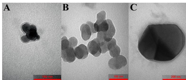
**Figure 2.** TEM images of A) chitosan nanoparticles, B) chitosan nanoparticles containing *C. verum* EO, and C) chitosan nanoparticles containing cinnamaldehyde
