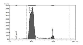
**Fig 7.** Chromatogram of <sup>99m</sup>Tc-DMSA obtained at pH 8.4 in triple solvent system showing peaks: at R<sub>f</sub>=0-0.1 for <sup>99m</sup>Tc-DMSA(III) & HR -<sup>99m</sup>Tc, at R<sub>f</sub>=0.5-0.6 for bound<sup>99m</sup>Tc-DMSA(V) and a small peak at R<sub>f</sub>=0.9-1 for free pertechnetate, TcO<sup>\*</sup><sub>4</sub>.
