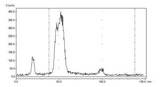
**Fig 6.** Chromatogram of <sup>99m</sup>Tc-DMSA at pH 5 in triple solvent system showing three peaks: one at  $R_{f}$ =0-0.1 for <sup>99m</sup>Tc-DMSA(III) & HR - <sup>99m</sup>Tc, the second small peak at  $R_{f}$ =0.5-0.6 indicates poor labeling of <sup>99m</sup>Tc-DMSA(V) while the third peak at  $R_{f}$ =0.9-1 shows free pertechnetate, TcO'<sub>4</sub>.
