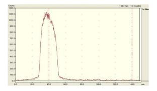
Fig 3. Chromatogram of  $^{99m}$ Tc Phytate indicating two peaks: one at R<sub>f</sub>=0-0.1 for the complex and other at R<sub>f</sub>=0.9-1 for free pertechnetate, TcO<sup>-</sup><sub>4</sub>.
