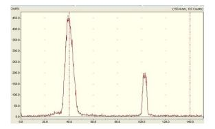
Fig 4. Chromatogram of  $^{99m}\text{Tc-DMSA}$  showing peaks: one at  $R_f\!\!=\!\!0.0.1$  for the HR  $^{-99m}\text{Tc}$  and the desired complex and the other at  $R_f\!\!=\!\!0.9\text{-}1$  for free pertechnetate, TcO $_4$ .
