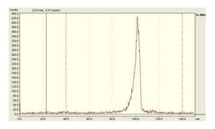
Fig 5. Chromatogram of  $^{99m}\text{Tc}\text{-}\text{DTPA}$  indicating peaks: one at  $R_f{=}0{-}0.1$  for the HR  $_{-}^{99m}\text{Tc}$  and the other at  $R_f{=}0.9{-}1$  for complex and free pertechnetate, TcO $_4.$
