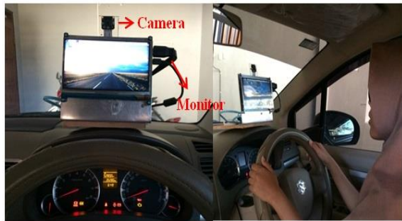
Fig. 3: Driver Drowsiness and Lost Focus Detection System
