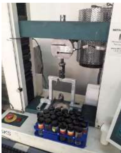
Fig. 1. Custom-made device for placement of bracket and wire sets in the universal testing machine
