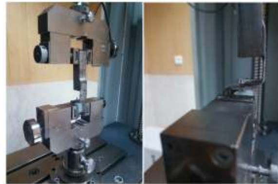
Fig. 4. Placement of specimens for pull-out test in the universal testing machine with load application at a crosshead speed of 1 mm/min
