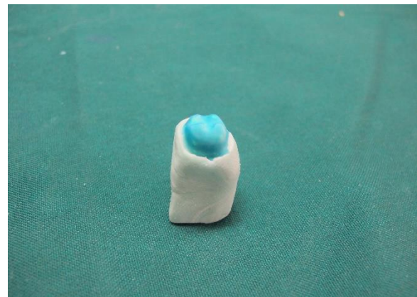
Fig. 3. The replica was made by condensation silicone
