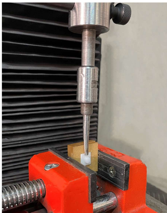
Fig 1. Applying Shear loads to the core-venearing interface in a universal testing machine
