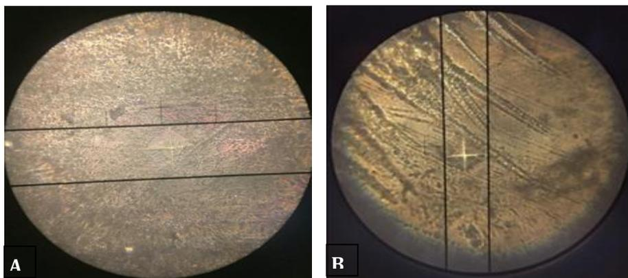
**Fig 2.** Microscopic images of the probe trace on (A) conventional, and (B) bulk fill composite surfaces
