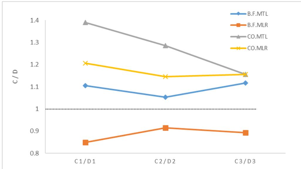
**Fig 4.** The C/D ratio of hardness at different depths for bulk fill (BF) and conventional (CO) composites with metal (MTL) and transparent (MLR) bands.
