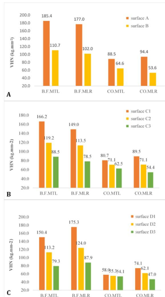
**Fig 3.** Microhardness in bulk fill (BF) and conventional (CO) composites with metal (MTL) and transparent (MLR) bands measured near A and B surfaces (chart A), adjacent to the matrix strip for C1, C2, and C3 surfaces (chart B), and D1, D2, and D3 surfaces (chart C)
