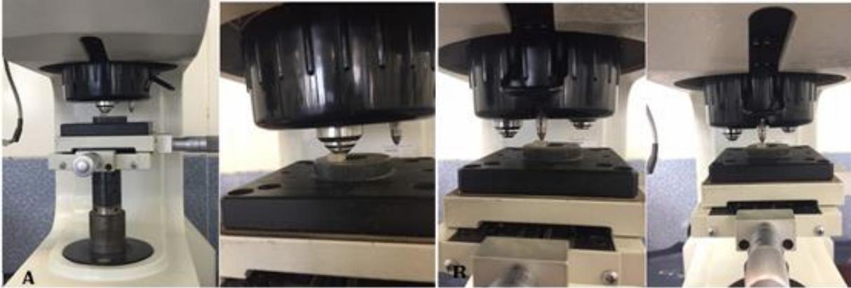
**Fig 1.** Microscopic evaluation of composite surfaces (A) and Application of force on the composite samples using a pyramid diamond probe (B)
