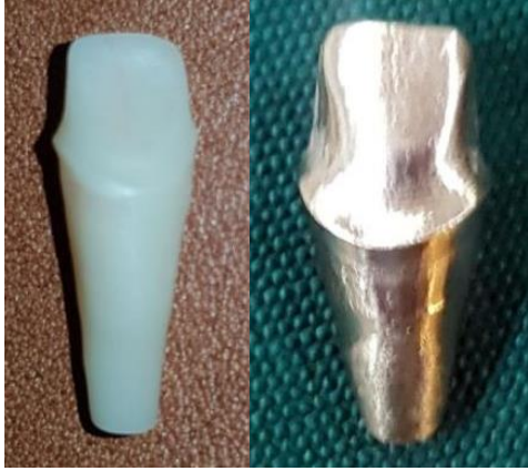
Fig. 3: Metal dies fabricated from premium chromium-cobalt. Left: Polymethyl methacrylate die; Right: chromium-cobalt die.
