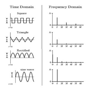
**Figure 4.** Time-domain and frequency-domain graphs of the square, triangle, rectified, and sin waves
