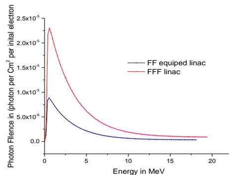
**Figure 2.** MC derived FF and FFF linac photon beam spectra. The photon beams spectra derived at 1m from the upward positioned linac for each FF
