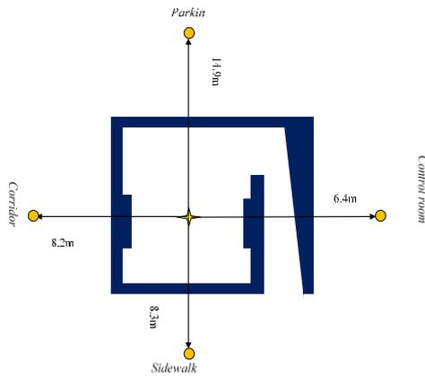
**Figure 1.** The schematic representation of the simulated 18MV linac treatment room and skyshine dose rate estimations by detectors at different distances from the X-ray source
