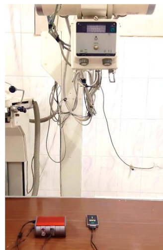
Figure 1. Measurement Setup; Barracuda package and Multi-Purpose Detector (MPD)
