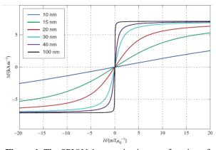
**Figure 1**. The SPIONs'magnetization as a function of magnetic field (H) and different diameters (D) in a given iron concentration [4]
