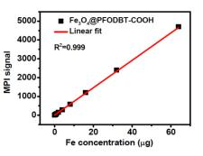
**Figure 4.** Linear correlation between MPI signal and Fe concentration ( $R^2$ =0.999). This correlation offers the exact quantification of the tracer [12]
