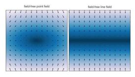
Figure 3. Schematic diagram of the selection gradient field for an MPI scanner based on a) FFP b) FFL. The dark blue and white colors represent the gradient field with zero strength and the maximum strength, respectively [4]
