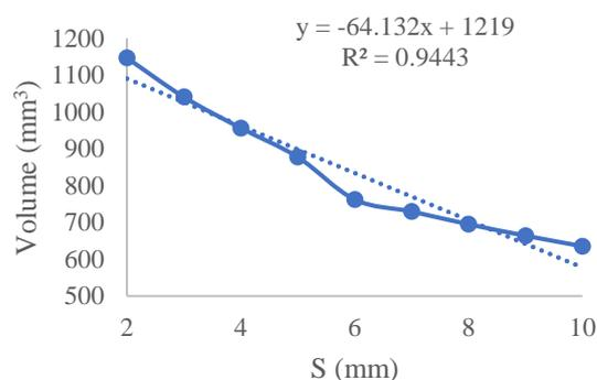
**Figure 6.** Effect of insulated pole length on tissue volume with cell killing probability >80%
