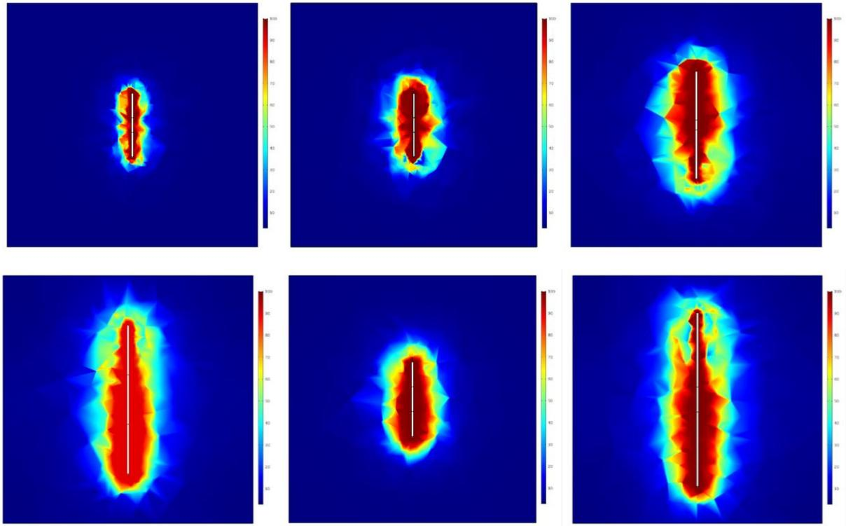
**Figure 7.** Impact of voltage, conductive pole length (P), and insulated pole length (S) on cell killing probability distribution inside the tissue. a- (P=5 mm, S=3 mm, V=700 V) b- (P=5 mm, S=3 mm, V=1500 V) c- (P=10 mm, S=2 mm, V=1000 V) d- (P=10 mm, S=10 mm, V=1000 V) e- (P=5 mm, S=5 mm, V=1000 V) f- (P=15 mm, S=5 mm, V=1000 V)
