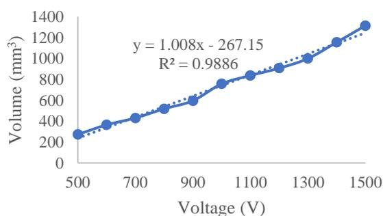
**Figure 4.** Effect of pulse voltage on tissue volume with cell killing probability >80%
