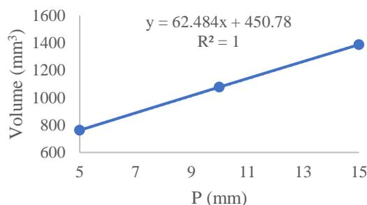
**Figure 5.** Effect of conductive pole length on tissue volume with cell killing probability >80%
