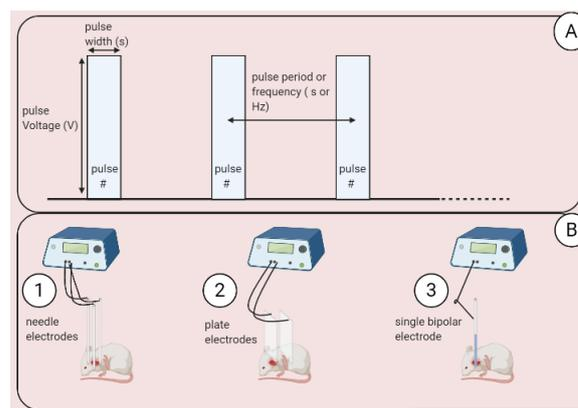
**Figure 2.** A) Electric pulse and their parameters B) different electrode 1- needle electrode 2-plate electrode 3-bipolar electrode
