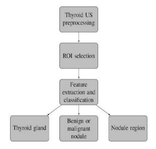
**Figure 2.** Block diagram of a typical CAD system for sonographic diagnosis of thyroid cancer
