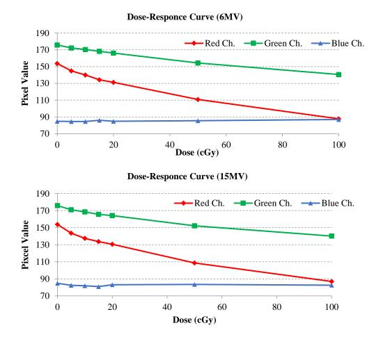
Figure 2. Response curves of radiochromic films exposed to different doses of LINAC in both energies for all three channels of the flatbed scanner
