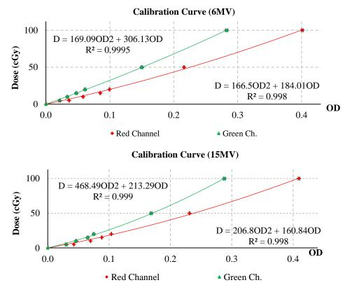
Figure 3. Calibration curves of radiochromic films exposed to different doses of LINAC in both energies in terms of OD versus dose for red and green channels of flatbed scanner
