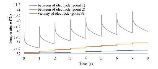
**Figure 4.** Temperature changes for candidate points (between electrodes, electrode margin, and the point between electrodes 2) per unit time for a pulse of 2000 V/cm with variable conductivity
