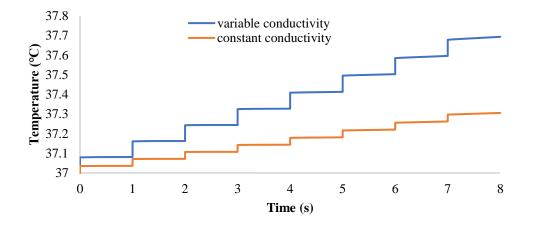
**Figure 7.** Temperature changes for points between electrodes (point 1) per unit time for a pulse of 3000 V/cm using variable conductivity and constant conductivity
