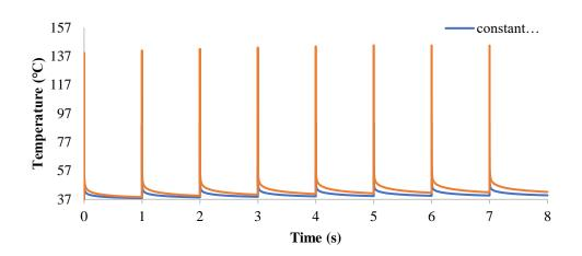
**Figure 6.** Temperature variations for electrode tip points per unit time for a pulse of 3000 V/cm using variable conductivity and constant conductivity
