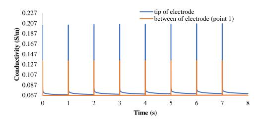
**Figure 3.** Conductivity changes per unit time for the electrode tip points and the point between the electrodes (point 1) for a pulse of 2500 V/cm
