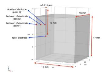
Figure 1. Geometry and candidate points used in this study
