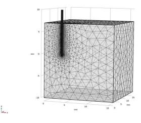
Figure 2. Geometry with the mesh
