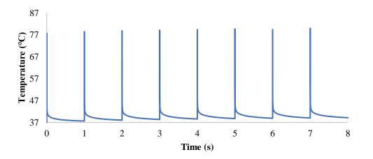
Figure 5. Temperature variations for electrode tip points per unit time for 2000 V/cm pulses using variable conductivity
