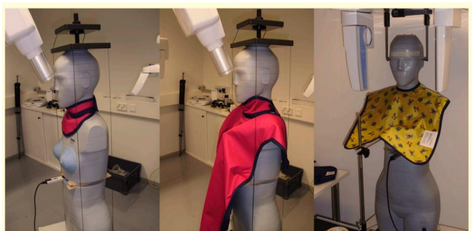
Figure 1. The shields were designed for three specific areas: (a) the thyroid, (b) the breast and abdominopelvic region, and (c) the breast and upper abdomen [20]
