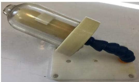
**Figure 2.** An in-house heart phantom to assessing image quality of the ProSPECT system
