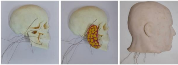
Figure 2. 3D-printed PLA skull model (left). 3D-printed silicone parotid gland replica and the live wire system (middle). Skin layer mold (right)
