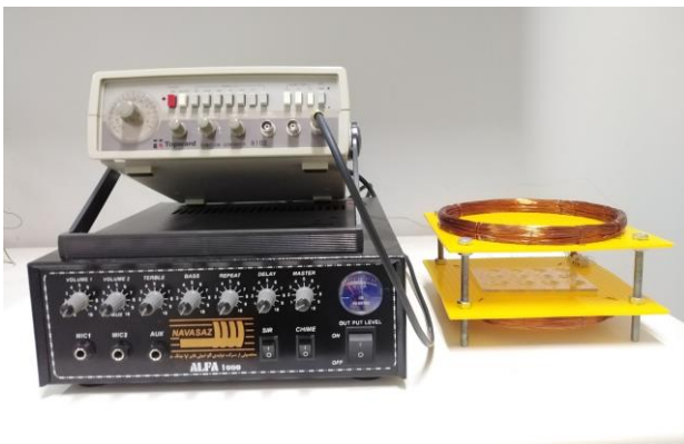
Figure 1. Experimental Electromagnetic Field (EMF) exposure set-up
