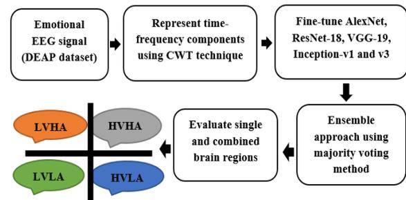
**Figure 2.** The flowchart of the proposed ensemble of CNNs for the recognition of four emotional states (HVHA, HVLA, LVLA, and LVHA) from EEG signal
