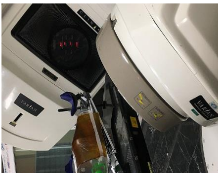
Figure 2. Irradiation of film dosimeters with 6 MV photons
