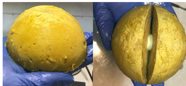
Figure 3. Oil-gelatin phantom of the breast
