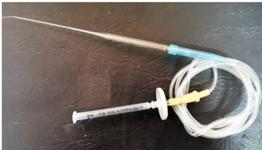
Figure 1. Mouth pipette used to harvest the granulosa cells after the ovaries punching
