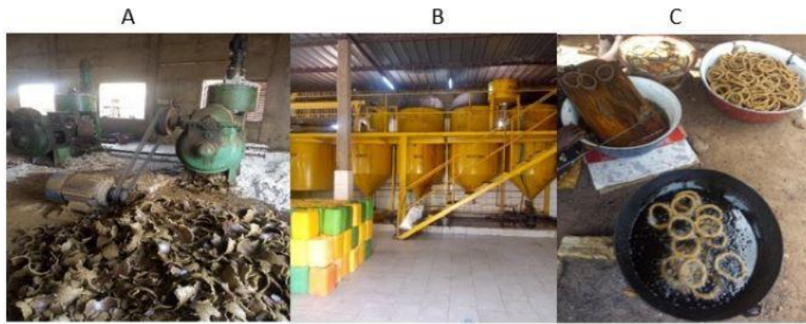
Figure 2. Materials used for producing and refining of the cottonseeds and crude peanut oils (A: Electric press for obtaining crude cottonseeds oil, B: tanks for refining the cottonseed oils, C: refining and frying of Koura-Koura by crude peanut oil).
