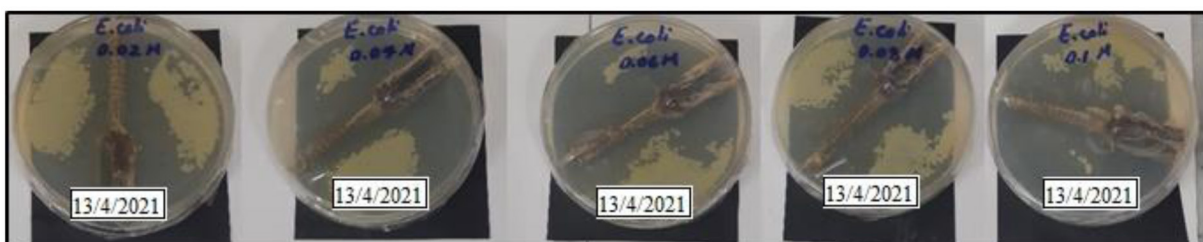
Figure 6. Antibacterial properties of silver-PVP composite-coated implants at different concentrations by deep coating method in the presence of E. coli bacterium.
