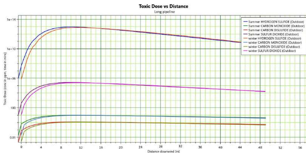
Fig. 2: Toxic dose vs. distance in wind direction for breach 20% scenario
