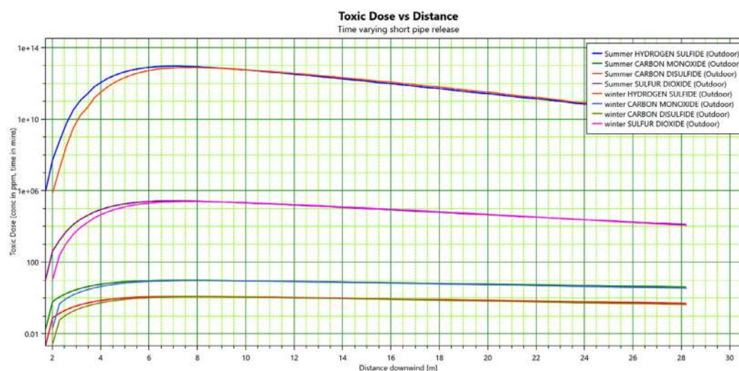
Fig. 3: Toxic dose vs. distance in wind direction for Time-Varying Short Pipe Release scenario
