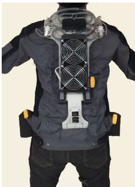
Fig. 3: A visual representation of the LCG as worn by the test subject
