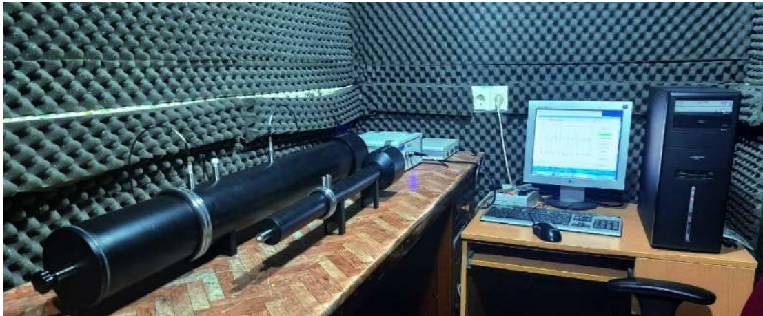
Fig. 1: Two-microphone impedance Tube setup
