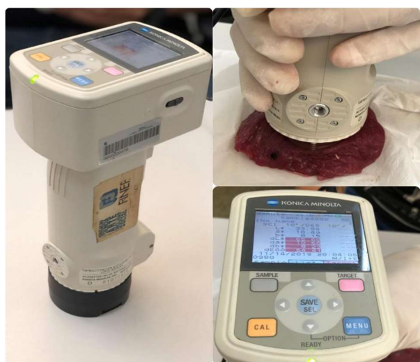
Figure 2. Minolta CR portable colorimeter (Chroma Meter CR-300, Konica Minolta Sensing Americas Inc., Ramsey, NJ).
