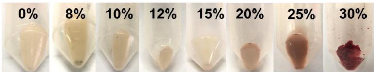
Figure A2: Cell pellets collected from inoculated YS^{+C,50ppm} medium including NaCl at different concentrations (0-30%) after 48 h of inoculation with K. quasipneumoniae GT7 and static incubation at 30°C.
