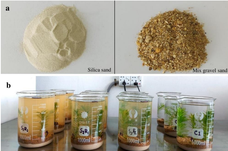
Figure 1: Pictorial plates of employed media (a), Experimental setup (b).
