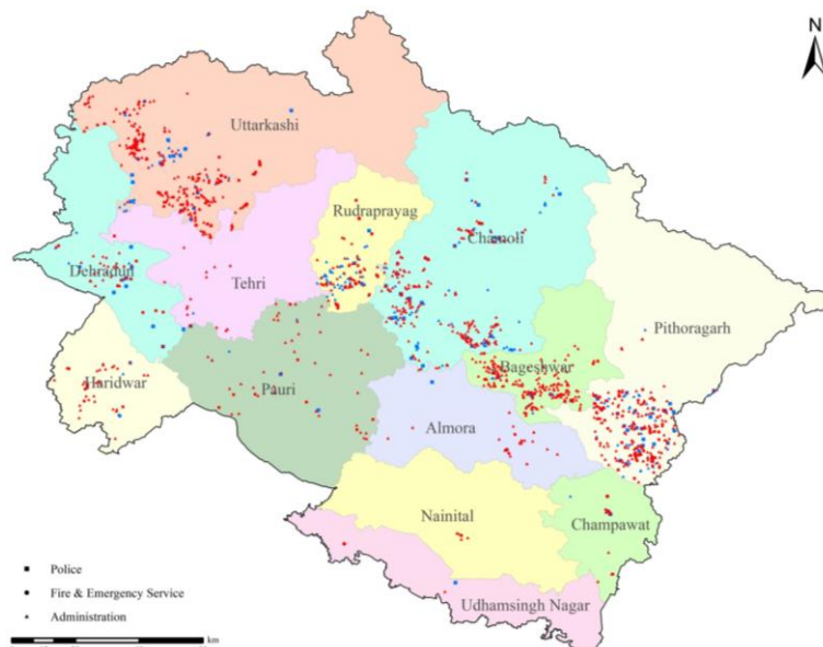
Figure 2. Spatial distribution of the surveyed buildings of local administration, Police and Fire, and Emergency Service (Masonry buildings are depicted in red and RCC buildings in blue)
