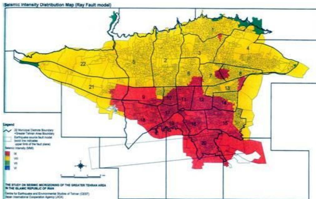
Figure 5. Earthquake Severity Dispersion Map- Rey Fault Model
