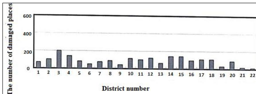
**Diagram 1.** The vulnerability of water supply pipelines in different districts of Tehran based on the floating model
