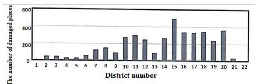
**Diagram 2.** The Vulnerability of water supply pipelines in different areas of Tehran based on Ray fault model
