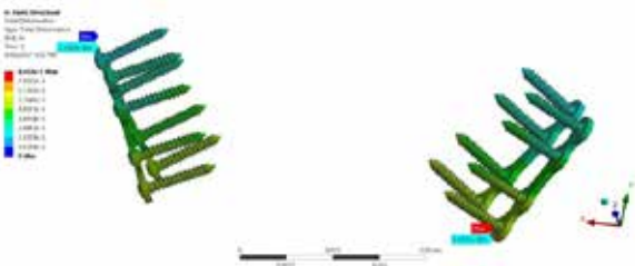
Figure 14. The Two-Parallel Fixation Method, Deformation Contours.
