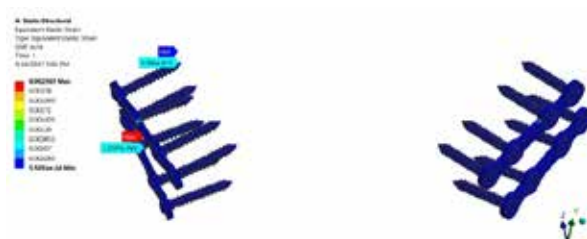
Figure 16. The two-parallel fixation method, strain contours.
