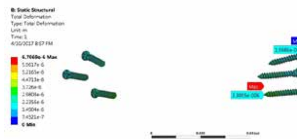
Figure 17. The triangular screw fixation method, deformation contours.
