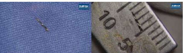
Figure 4. Retrieved fragment measured approximately 3.8 mm in length following removal.
