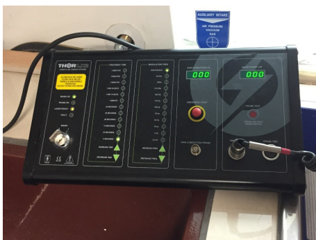
Figure 2. Low-level diode laser (THOR Photomedicine Ltd, UK) with wavelengths of 660nm and 810nm.
