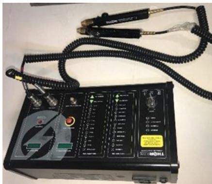
Figure 3. Laser of red 660 nm (THOR Photomedicine Ltd, UK), and Infrared 810 nm (THOR Photomedicine Ltd, UK) wavelength.
