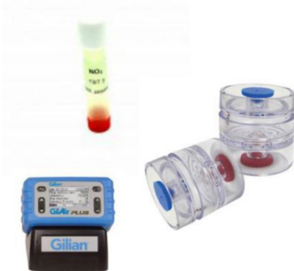
Fig. 2. NO 2 and PM 2.5 sampling devices
