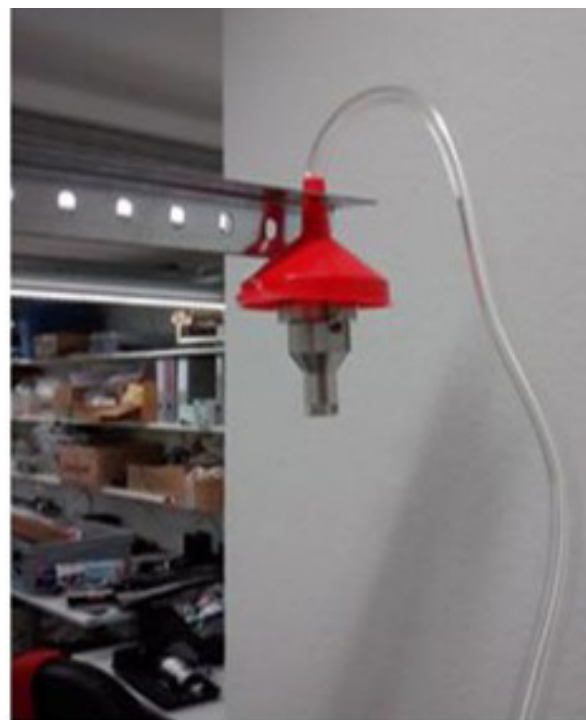
Fig. 2. NO 2 and PM 2.5 sampling devices
