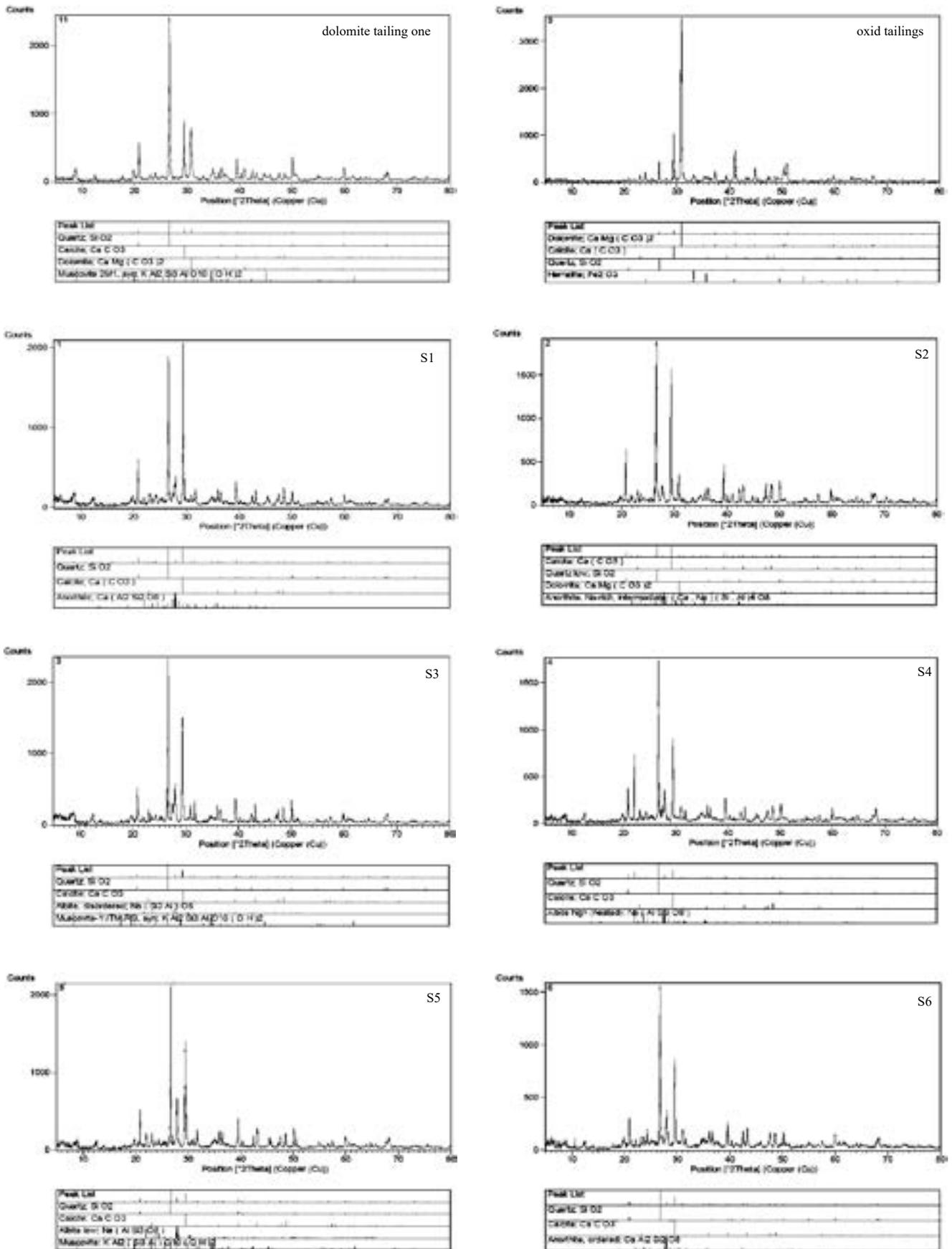
Fig. 6. display of Mineralogy characteristics of the dust particles by XRD
