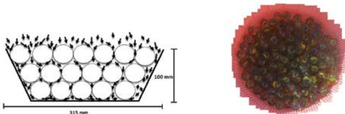
Fig. 2. MDCO samplers used in order to collect the falling dust
