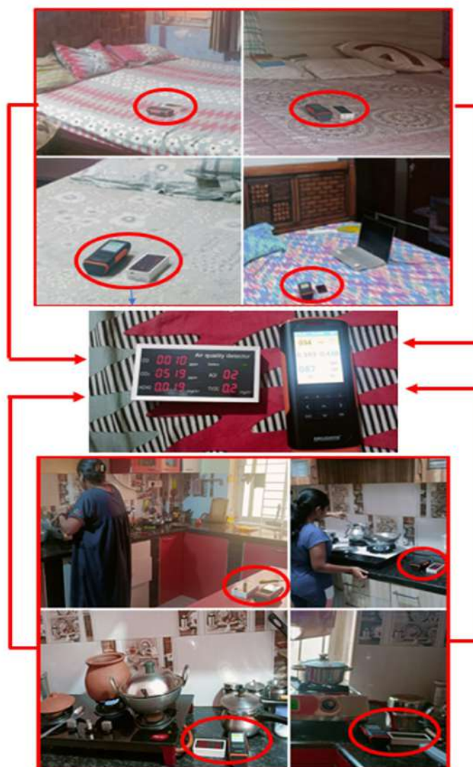
Fig. 4. Sample photographs of bedrooms and kitchen during the measurements with the help of air quality monitor
