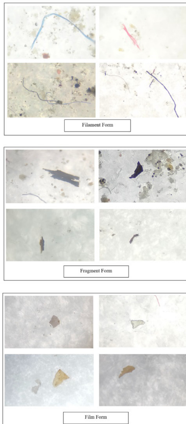
Fig. 6. Microplastic forms of filaments, fragments, and films with observation under a microscope
