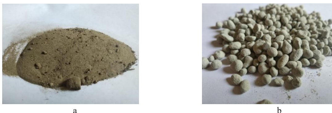
Fig. 1. a) Fly ash as Powder form; b) Fly ash as Pellets form
