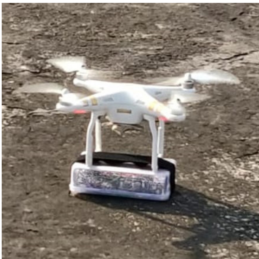
Fig. 3. UAV with sensor based air quality monitoring systems
