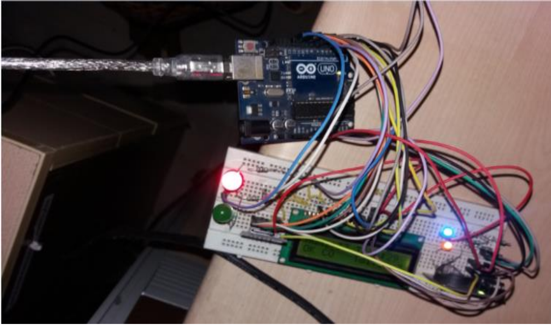
Fig. 5. Receiver section consisting of LEDs indicator for sensors
