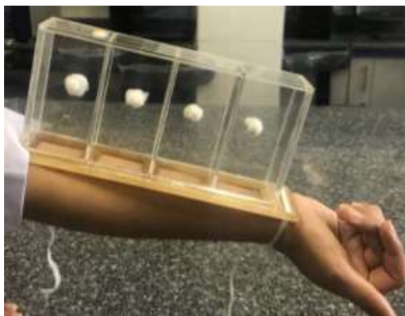
Fig. 1. Modified 4-celled Klun and Debboun module used for the repellency assay of dichloromethane (DCME-TP) and ethanolic extracts (EE-TP) of T. polium against Anopheles stephensi
