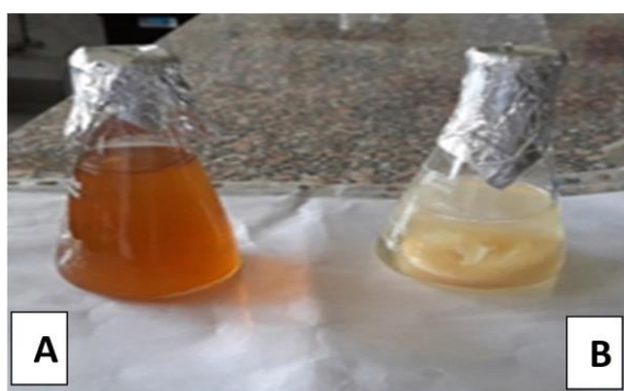
Fig. 1. (A) Color change from yellow to dark brown of aqueous solution filtrate of Penicillium fungus after treatment with \text{AgNO}_3 . (B) Shows a flask of fungal biomass in aqueous solution.
