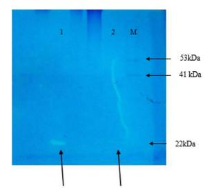
**Fig. 2.** The results from zymogram tests were confirmed the enzymatic activity of the protein with a mass of 22 kDa. line1. partially-purified CFS Lys46; line2. CFS Lys46; M. Size Marker proteins 10-170 kDa. The arrows are showing the digestion of cell wall.
