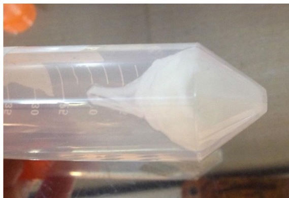
Fig. 1. W. confusa B4-2 EPS precipitated in ethanol
